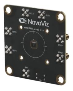
The sensor combines the benefits of a single-photon avalanche diode (SPAD) pixel, namely the single-photon resolution and fast operating speeds, with the benefits of on chip timestamping and memory – high event rates and reduced output data rates.
