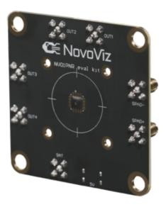
The sensor combines the benefits of a single-photon avalanche diode (SPAD) pixel, namely the single-photon resolution and fast operating speeds, with the benefits of on chip recharge and threshold circuitry – high event rates and reduced noise.
