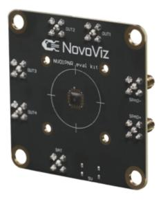
The sensor combines the benefits of a single-photon avalanche diode (SPAD) pixel, namely the single-photon resolution and fast operating speeds, with the benefits of on chip digital processing – reduced output data rates.
