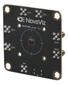
The sensor combines the benefits of a single-photon avalanche diode (SPAD) pixel, namely the single-photon resolution and fast operating speeds, with the benefits of on chip recharge and threshold circuitry – high event rates and reduced noise.
