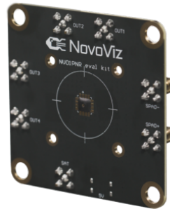
NV02TPX-DEV Two- pixel correlator development module
