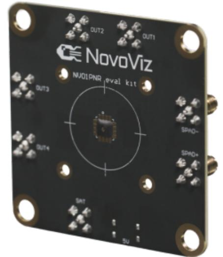
The sensor combines the benefits of a single-photon avalanche diode (SPAD) pixel, namely the single-photon resolution and fast operating speeds, with the benefits of on chip timestamping and memory – high event rates and reduced output data rates.
