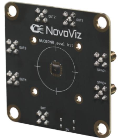
The sensor combines the benefits of a single-photon avalanche diode (SPAD) pixel, namely the single-photon resolution and fast operating speeds, with the benefits of on chip digital processing – reduced output data rates.
