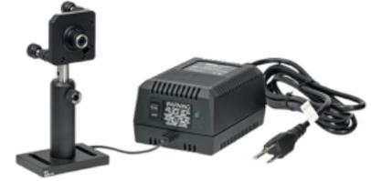
This class 3R visible laser emits at 635 nm and can be finely adjusted for precise positioning via adjustment actuators with the supplied kinematic mount.
