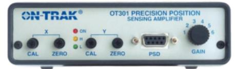
The OT-301 Position Sensing Amplifier is the easiest, most precise way to process the current output from any position sensing detector (PSD) on the market.
