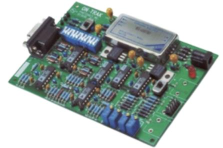
Precision op amps and precision resistor networks provide the final ratio. The analog dividers provide the utmost in linearity over a very wide signal range.
