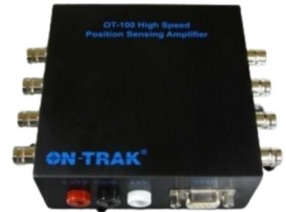
The OT-100 is designed to output bipolar voltages representing the position and intensity of a light spot on the PSD at bandwidths of up to 400 kHz. BNC outputs allow simple and fast connection to voltmeters and oscilloscopes. Banana jacks are provided for easy connection to most common power supplies. Plug and play connection to PSM modules and PSDs are made via the DB9 input and supplied DB9 cable.
