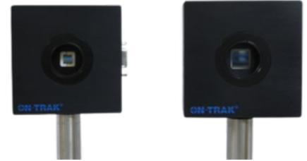
The PSD outputs bipolar voltages representing the position and intensity of the centroid of a light spot on the PSD at bandwidths up to 400kHz. Inputs are available for external adjustment of offset voltages. The SPC PSM is offered in a variety of one dimensional or two dimensional sizes.
