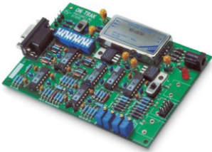
OT-301DL - Position Sensing Amplifier For Duolateral PSDs
