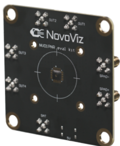
NV07SLN-DEV Small line sensor development module
