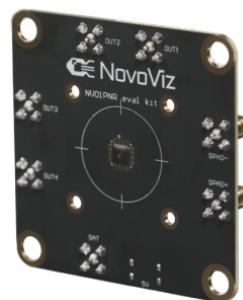
NV01PNR-DEV Photon number resolver development module
