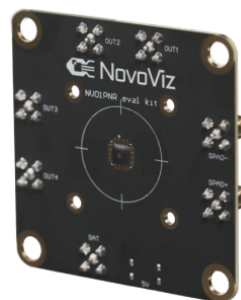
NV01PNR-DEV Photon number resolver development module
