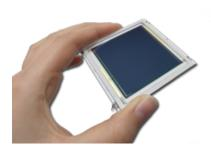
There is also an UV version available. The UV PSD is a detector optimized for use in the UV wavelength region 200-400 nm, although its spectral response reaches up to 1100 nm. The sensitivity in the UV region (200-400 nm) is extremely high. The UV-PSD has the same outstanding specifications as the standard SiTek PSD.
