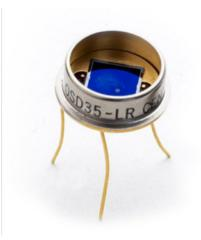
The detectors offer high responsivity in the 800-1000 nm range but are equally suited to high speed application at longer wavelengths where maximum absolute responsivity is not as important as speed of response.
